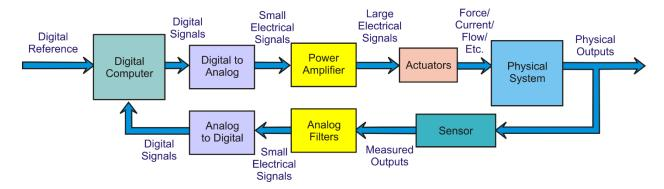
If we take a "walk around the loop" in this diagram, we discover a large set of pieces that need to be "gotten right" in order for the physical system to be properly controlled. Often, these blocks have not been discussed since the second week of the first undergraduate controls class. Specifically, we will first visit:
