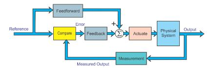
This section will discuss practical application of feedforward control to a feedback loop. In large part, feedforward can remove a lot of the potential error from the control loop,
