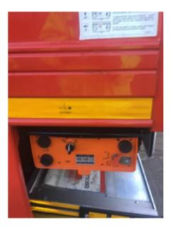
• To deploy the tail lift platform, lower the tail lift platform using the lower control button (LOWER) following the operator instructions, fully deploy the tail lift platform out using the out control button (OUT) checking the area for pedestrians throughout.
