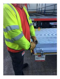
• Hinge out the tail lift flaps by gripping the hand hold and raising it to the vertical with both hands. Then lift the flap to free it from its stops and lower until it reaches its horizontal stop. Repeat this process with the other flap.
