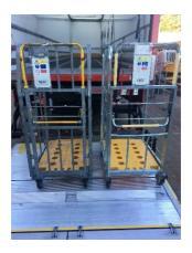
Loads must not exceed the tail lift Safe Working Load (SWL) of 1250kgs for Rigid Vehicles and 1500kgs for Trailers.
