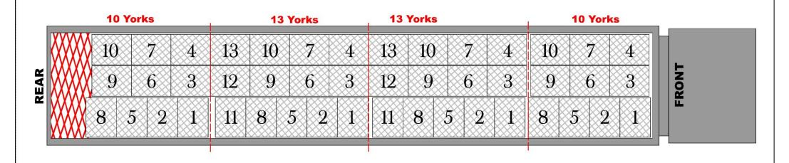
13.6m Straight Frame Double Deck – Lower Deck - With Internal Rubbing Rails (Trailer Internal Dimensions: Width 2378mm x Length 13305mm) Moving Deck – Width 2265mm x Length 13067mm
