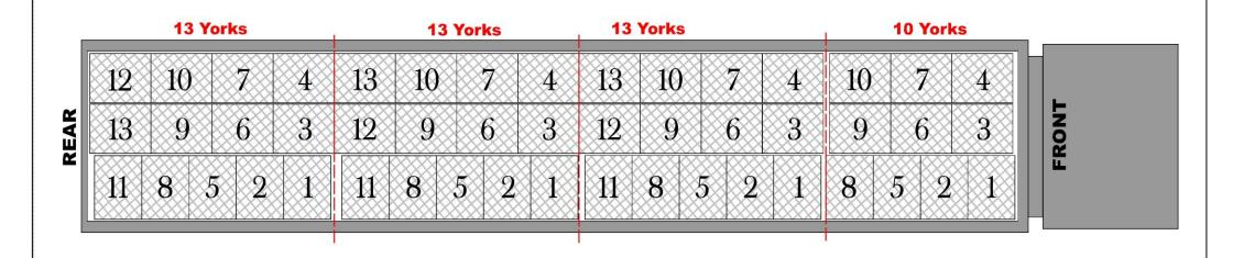
13.6m Straight Frame Double Deck – Lower Deck - With Internal Rubbing Rails (Trailer Internal Dimensions: Width 2378mm x Length 13305mm) Moving Deck – Width 2265mm x Length 13067mm
