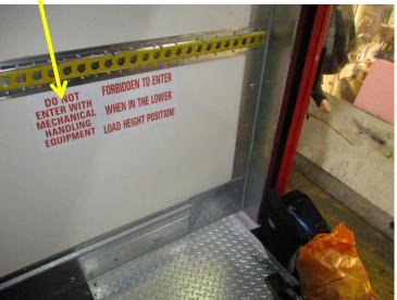
Lower deck - N/S/R panel and O/S/R panel revised decals fitted
