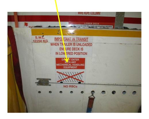
Moving deck – N/S/R Open gate and O/S/R Open gate revised decals fitted (please ensure the bi-fold gates are closed as pictured and the decals fitted so they are clearly visible when in this position).
