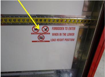
Moving Deck – N/S/R decal to be removed – not all trailers have the same decal fitted on the O/S/R panel but if there is one this MUST be removed as well.
