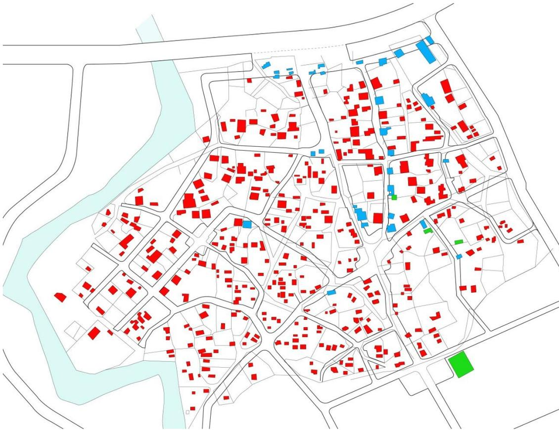
**Fig. 4.58:** Proposed plan for a rationalised Junawada before the earthquake. The red blocks indicate the location, size and approximate shape of the original buildings that would be reconstructed or renovated; the blue blocks indicate buildings that would have to be removed to make way for the proposed new road layout (heavy black lines); the lighter black lines indicate the original positioning of property and road boundaries.
