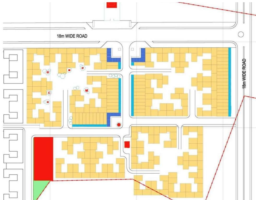
**Fig. 4.15:** Detail of Master Plan (Fig. 4.14, above) ~ Clusters. The ODR cluster housing approach appears to be systematic insofar as it promotes a set of typologically appropriate and more-or-less identical basic ‘core units’, designed to invite appropriation and alteration. The designer in this approach provides a ‘structural framework’, a flexible architectural and urban context.
