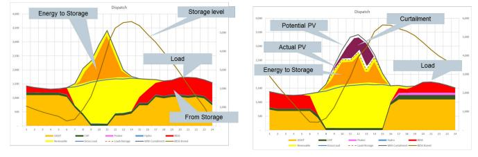
Figure 2: Timing of energy storage charging curtailment impacts
