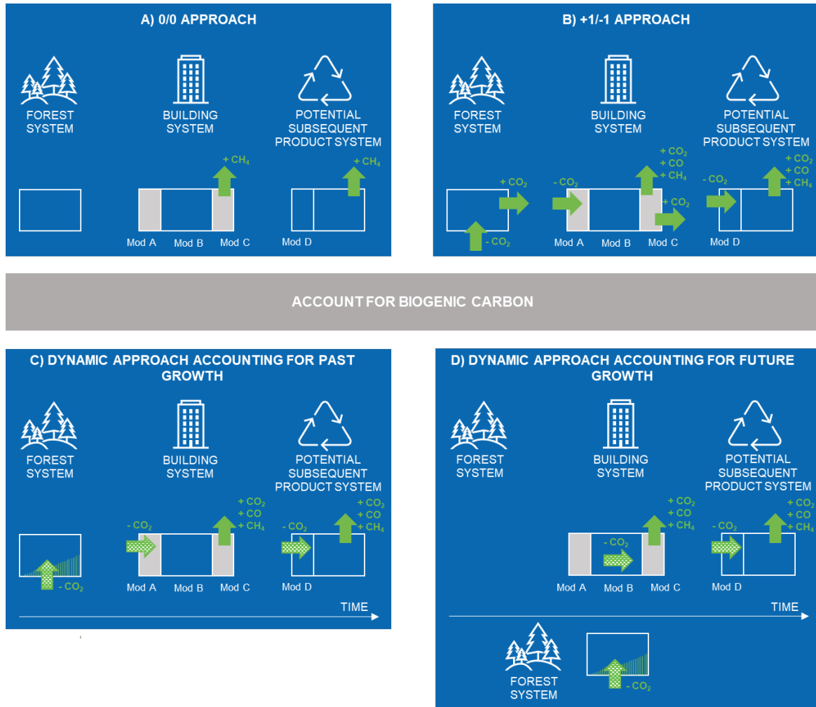
Figure 7: Overview of approaches to account for biogenic carbon uptake and release Source: Adapted from Hoxha et al. (2020)
