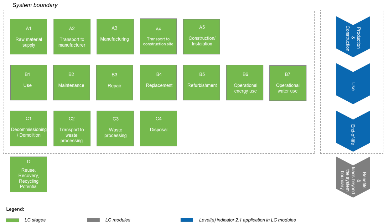
Figure 9: Bill of quantities and lifespan application in the context of the Life cycle stages Source: Adapted from EN 15804 (CEN/TC 350 2019)
