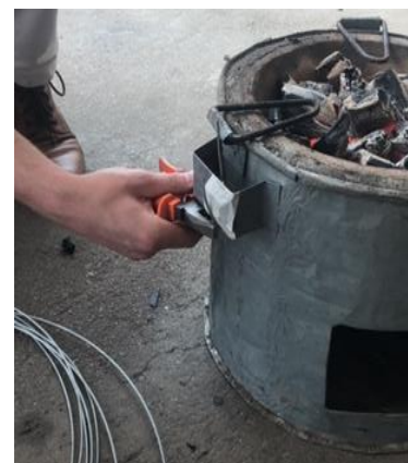
Figure 6: SUM being attached to charcoal stove. Photo credit: T. Perros
