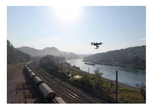
In response to these challenges, Infrabel has invested heavily in automating a number of maintenance processes. It's become exceptionally strong in developing innovative condition monitoring tools and it's recently been experimenting with drones to inspect the rail infrastructure. Drones are currently used mainly to control GSM-R masts.
